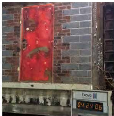
After Test Exceeded 4 Hours 24 Minutes
